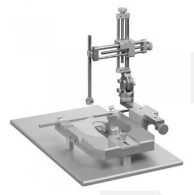
With 3-dimensional manipulator, ear bars and base plate
